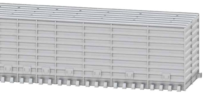
The scheme shows like a cell is built. All elements are zinc-coated, without wood-parts and are screwed together. The arrows show the air-current.
