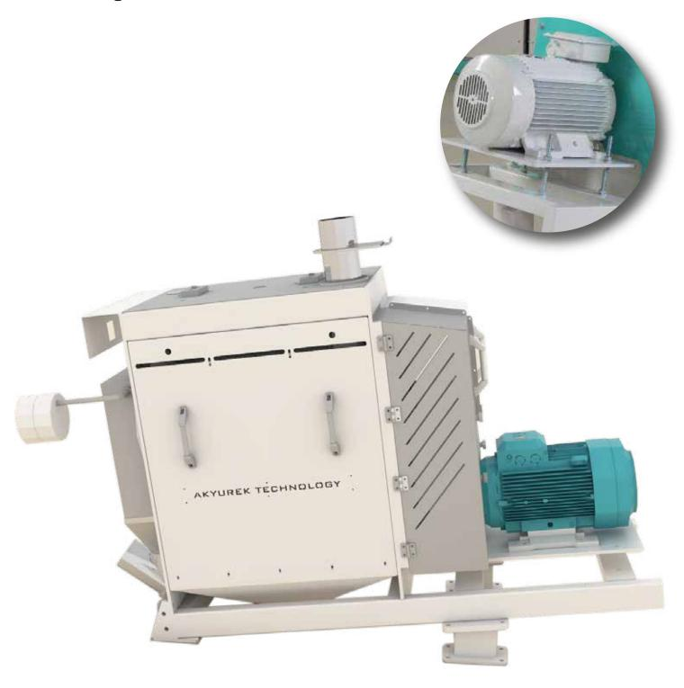
With Puls Hull & Split Akyurek is setting new standards in pulses processing. PHS 460 is an ideal machine for hulling (removing the seed coat) from pulses. -PIGEON PEA, CHICK PEA, BLACK GRAM, GREEN GRAM, YELLOW GRAM, YELLOW LENTILS, RED LENTILS
